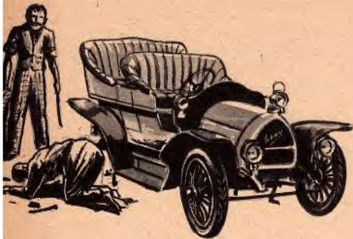
Mending a puncture. Once wheels were made detachable, mending a puncture became a much easier job.
